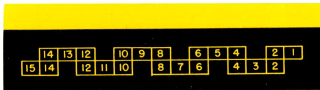
Fig. 6: This diagram shows how the eight filters, 200 MC wide, overlap each other by 67 MC, to cover the entire 1000 MC band.
