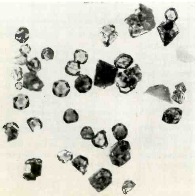
Fig. 2: Beautifully formed diamond crystals when viewed under a microscope range in color from dark green to pure white. Diamonds, excellent semiconductors, were formed at about 80,000 atmospheres and 1700° C.
