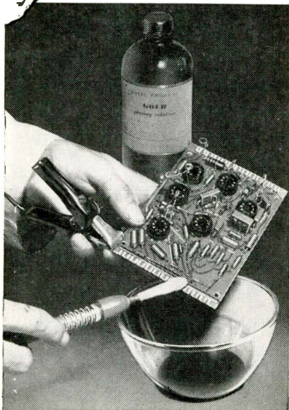
Plating circuit contacts without dismantling electronic components.
